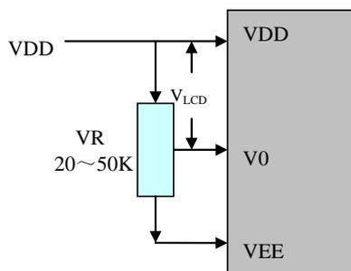
Note: Adjust V0 to VSS as an initial setting. When the module is operational, readjust V0 for optimal display appearance.
