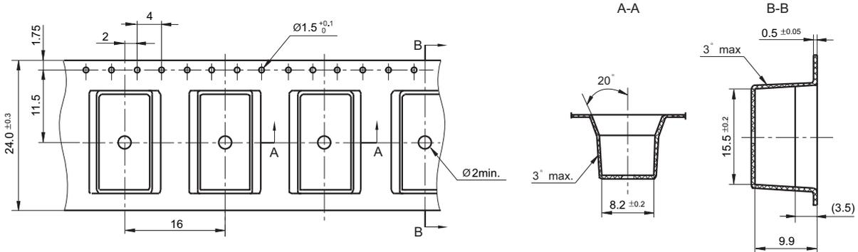
Remark: 1) In case of no tolerance shown in outline dimension: outline dimension  $\leq 1\text{mm}$ , tolerance should be  $\pm 0.2\text{mm}$ ; outline dimension  $\leq 5\text{mm}$ , tolerance should be  $\pm 0.3\text{mm}$ ; outline dimension  $> 5\text{mm}$ , tolerance should be  $\pm 0.4\text{mm}$ .
