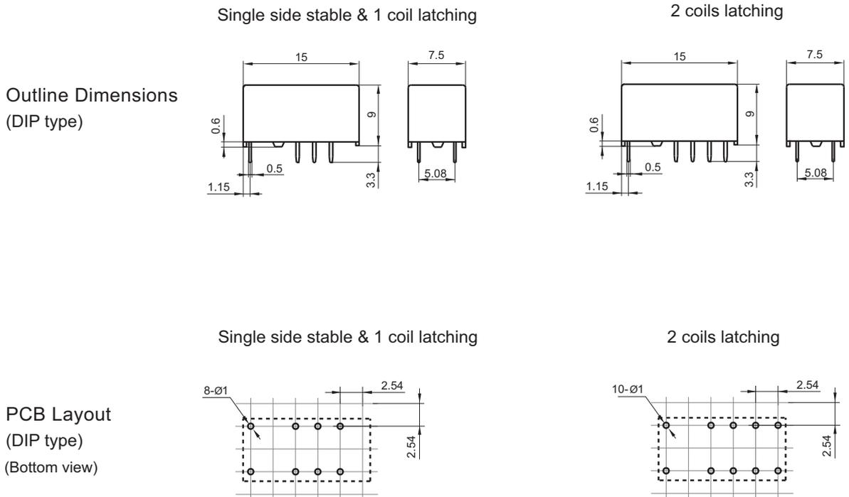
**OUTLINE DIMENSIONS, WIRING DIAGRAM AND PC BOARD LAYOUT**
