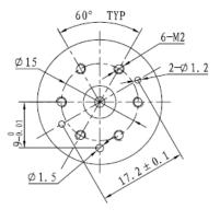
Usable machine screw length 1.5mm max. from motor mounting surface **Performance Curve:**
