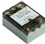
HHG3E-3 with Thermal protection (The SSR will shut down when the temperature of the base  $\geq 75^{\circ}\text{C}$ )
