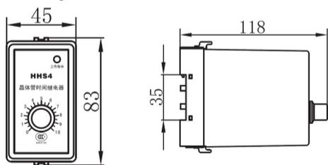
Surface mounting, DIN Rail mounting
