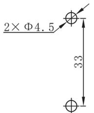
Installation of Flush mounting
