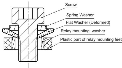
When use M5 screw, the thickness and strength of the washer needs to be guaranteed or it may deform and burst the cover.
