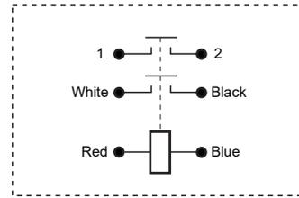
Note: No polarity on the load, auxiliary contacts and coil sides.
