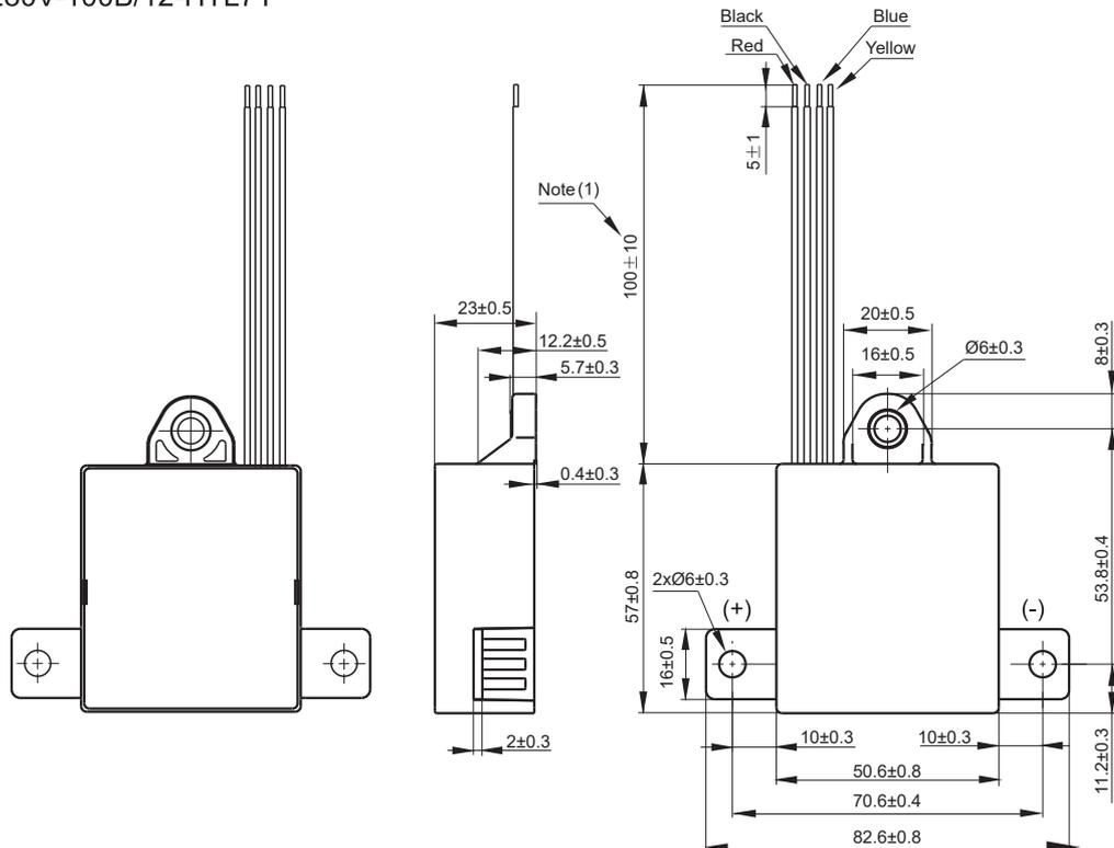
Note:1)The length of lead wire can be customized according to actual needs. If there is no special description,the default length of our company is 100mm.
