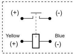
Note: Both the load side and coil side have polarity.
