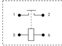
Note: No polarity on the load and coil sides.
