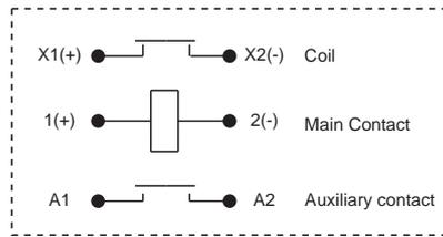
Note: Both the load and coil sides have polarity.
